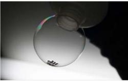
This is probably so far the most light-weight and tiny solar cell ever existed, so small and flexible that it can stay on top of a soap bubble without popping it. This ground-breaking idea came about when researchers realized that they can use a single process to produce the solar cell, the protective substrate and the overcoating. You can also check-out the original research paper published in Organic Electronics.
